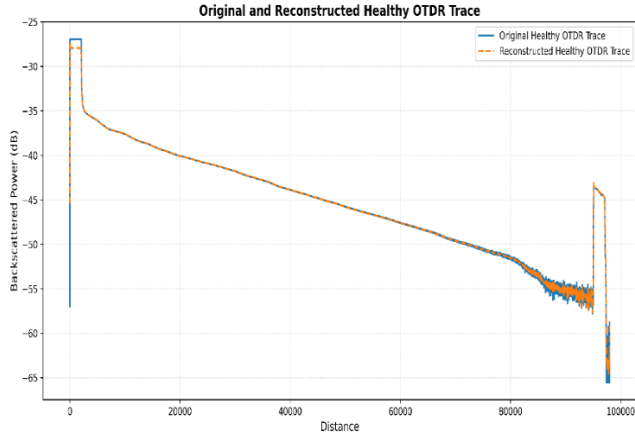
Fig. 4: Original and reconstructed healthy OTDR trace obtained using the trained convolutional autoencoder.
