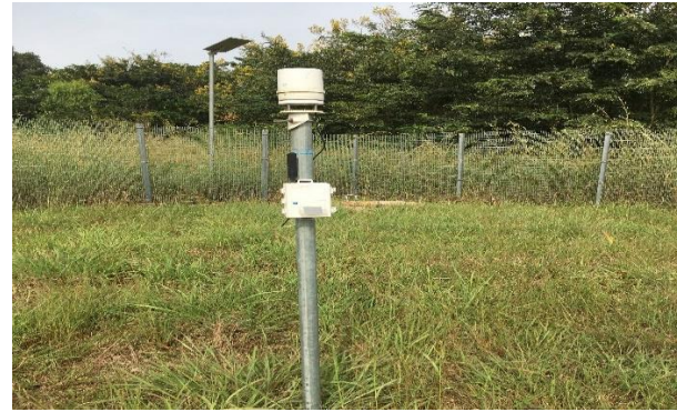
Figure 1: Automatic rain measuring setup powered by Em60G™ datalogger
