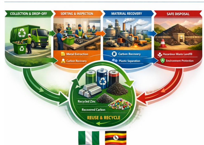
Fig. 4: Circular end-of-life flow for spent Zn-C batteries showing collection, sorting, material recovery and safe disposal in both countries
