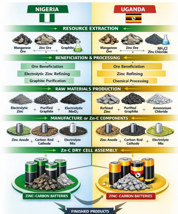
Fig. 2: Comparative Nigeria-Uganda Zn-C battery raw-material value chain and beneficiation pathway)
