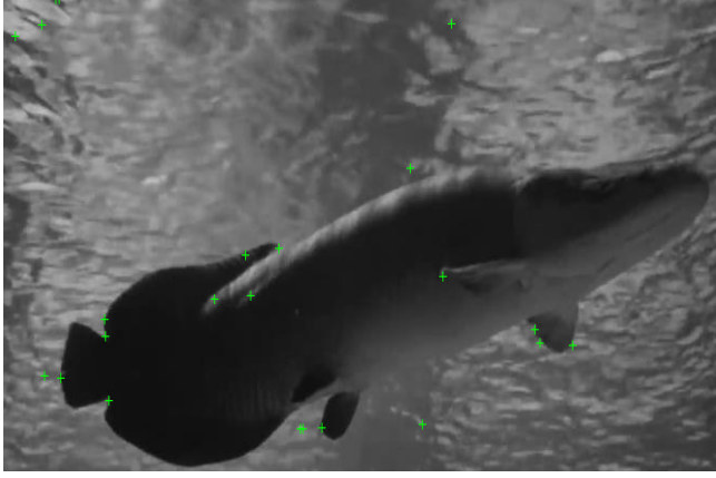
Figure 4 Corner Features of Arapaima Detected using FAST
