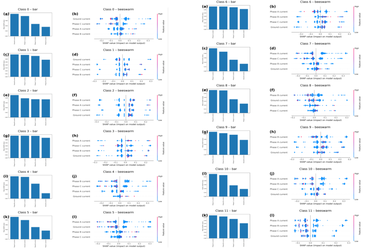
Fig. 6: Random Forest SHAP interpretation. Combined bar and beeswarm plots for classes 0–11 summarizing global feature importance and local contributions of Phase A, B, C and Ground currents to the RF decision function.
